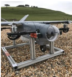
Figure 2 | Marble fixed wing BVLOS UAV.
